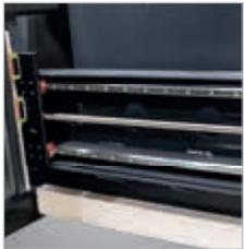
▶ The ball screw driven X axis is borne by double linear guides
