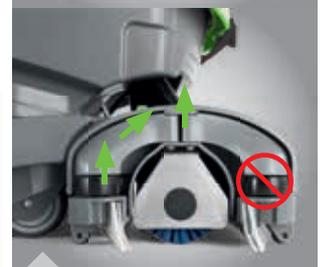
Extraction unit with dual, alternating extraction (**patented**). Water is taken up during **forward** and **reverse** motion
