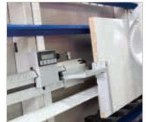
▶ Digital dimension display for length adjustment during vertical cutting
